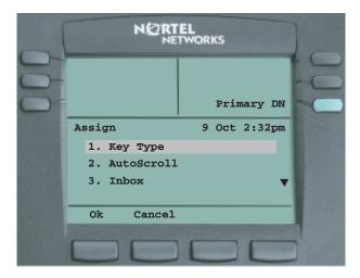
3. Press **Ok** to access the following screen in which you can assign the key type or press **Cancel** to return to the Feature menu:
